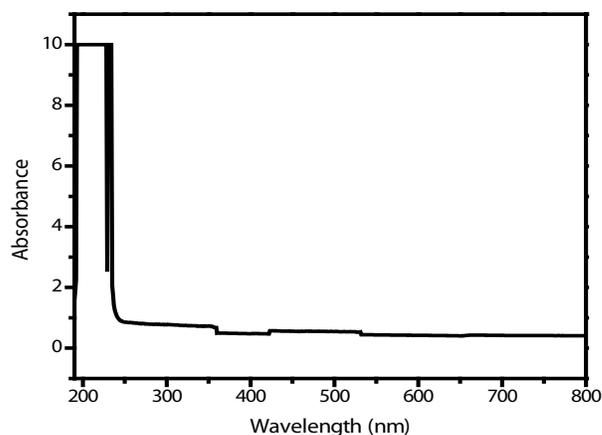
Fig.3: Absorption Spectrum of  $\gamma$ -glycine
